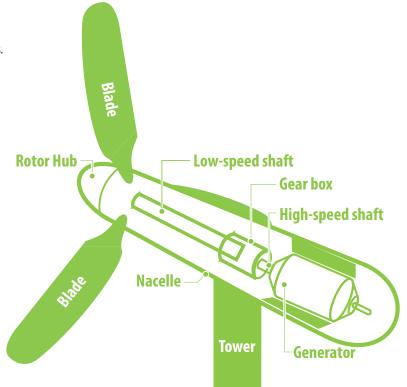
Large turbines can generate anywhere from 1 - 15 MW of power each. A group of turbines is called a wind farm. Offshore wind turbines are the largest turbines that often use a direct drive design where no gearbox is needed—just blades turning a generator.
