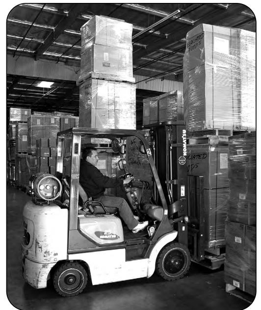
This forklift is fueled by propane.
