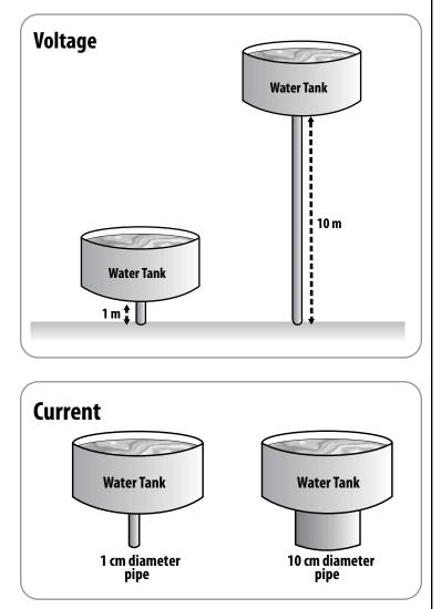
two points having a difference in voltage. Current is measured in **amperes** or **amps (A)**. One ampere is 6.25 X 10<sup>18</sup> electrons per second passing through a circuit.
