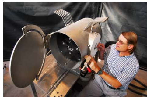
Above, Sandia researcher Rich Diver assembles a prototype device intended to chemically reenergize carbon dioxide into carbon monoxide, which could ultimately become the building block to synthesize liquid combustible fuels. Photo Credit: Randy Montoya.
